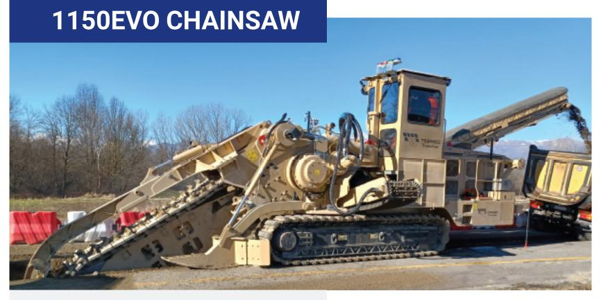
The Tesmec 1150 EVO Chainsaw Trencher is a specialized machine meticulously crafted for trenching tasks, particularly tailored to serve midsize pipelines and underground utilities.
