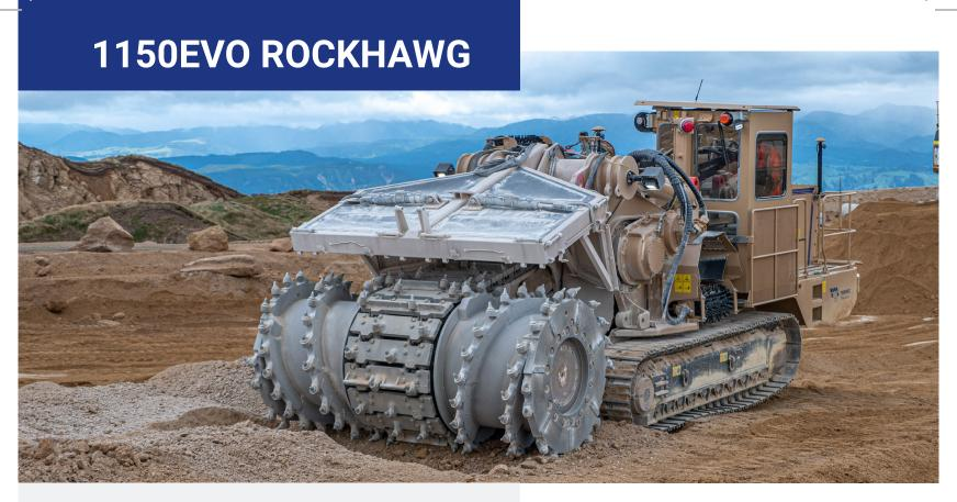
The 1150 EVO Rock Hawg represents a distinct adaptation of the EVO model, meticulously customized for uninterrupted surface mining endeavors. Its expansive 10'6" wide drum excels in bulk-excavation projects, open-pit quarries and mining operations.
