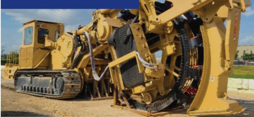
Tesmec 1475XL EVO Bucket wheel is a high performance 90 metric ton-class trencher featuring a 630 HP (470 kW) engine ideal for mid to big size pipelines projects in dirt and light rocky soils
