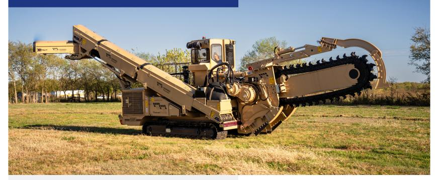
The Tesmec 950R Chainsaw stands as a mid-size, high-performance tool renowned for its exceptional precision and efficiency in a variety of jobs, ranging from laying fiber and utility lines, to including water, sewer or gas
