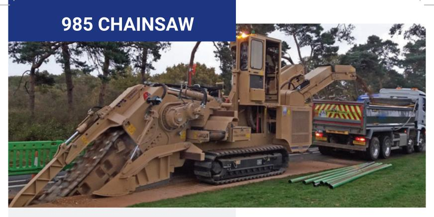
The Tesmec 985 Chainsaw (shown with a boom attachment) is a mid-size self-leveling offset trencher designed to cater to a diverse customer base, spanning from highway and pipeline contractors to those engaged
