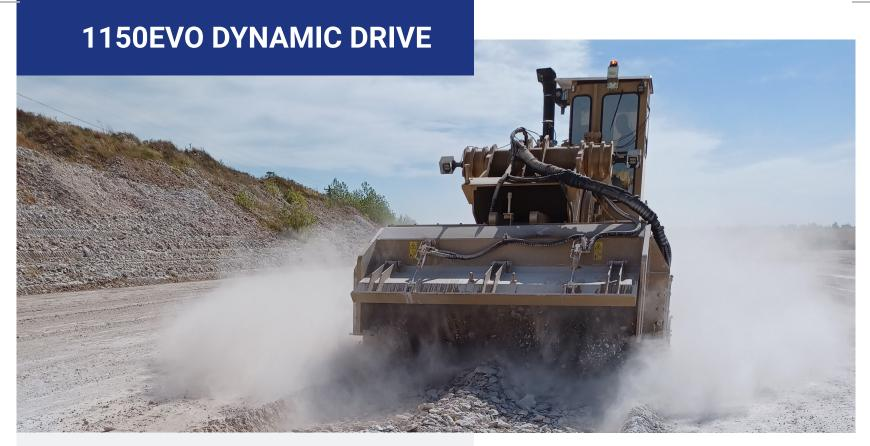
Tesmec 1150EVO Dynamic Drive is a 55 metric ton-class surface miner, featuring a 451 HP (336 kW) Tier 4/Stage V engine, or a 440 HP (328 kW) Tier 3 engine, employed in the surface mining of weak to medium-hard rock
