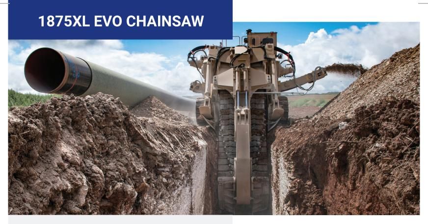
Tesmec 1875XL EVO is the largest 160 metric ton-class trencher and the most powerful featuring a 950 HP (709 kW) engine, designed for big diameter pipelines in hard rock and in the toughest excavating conditions
