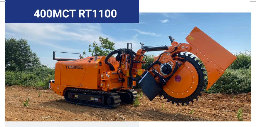
The Tesmec 400MCT – with its tangential wheel – stands out as a high-performance wheel trencher. The design caters to the demands of long-distance trenching for fiber optic, electric cable and small diameter water pipeline projects, whether situated in urban or rural environments.
