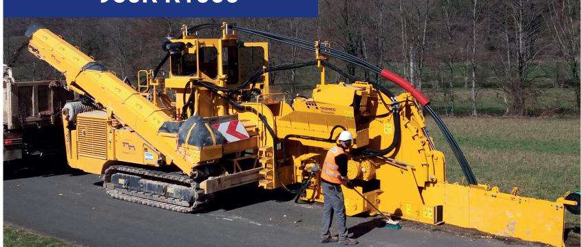
Tesmec 950R R1000 is a 27 metric ton-class trencher featuring with 275 HP (205 kW) engine designed for underground network projects in urban areas
