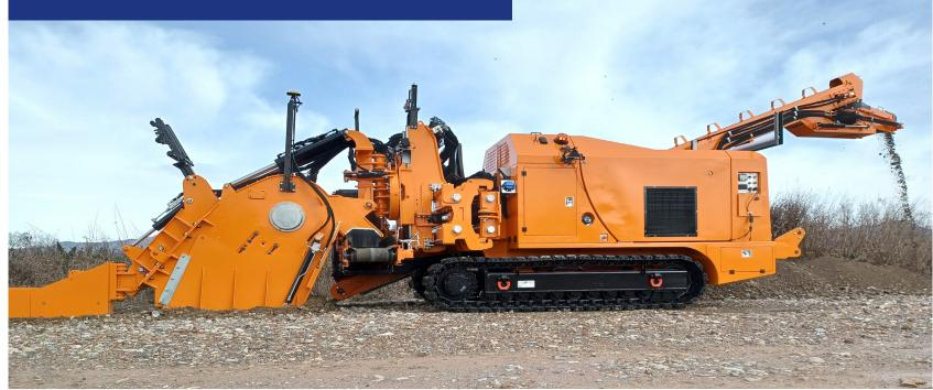
Tesmec 400MCT with CS1200 is a 15 metric ton-class trencher featuring a 238 Hp (175 kW) tier 4 engine/ Stage V, or a 218 Hp (160 kW) tier 3 engine, designed for telecom and energy cables projects in urban and extra-urban areas
